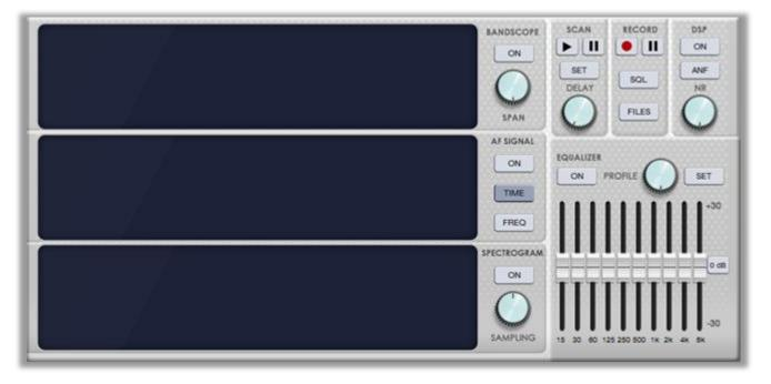
The left part of this interface allows the user to graphically visualize the band scope and audio output. The right part includes additional audio control functions and utilities.
