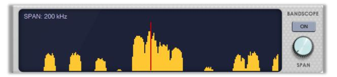
The band scope functionality of *PCR AnyWhere* works on the frequency domain of the received RF signal. In this mode, the band scope function sweeps in the specified span around the tuned frequency allowing the user to visually check the received signal strength on its display.
