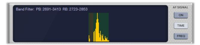
The upper text shows the bands in Hz covered by the pass band filter (PB) and the reject band filter (RB).
