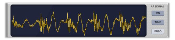
**PCR AnyWhere** has an embedded signal analyzer for the audio output signal. This analyzer is capable to represent the audio signal in the time domain, as represented above, or in frequency domain, as in the figure below. The representation mode is selected using the buttons '*TIME*' and '*FREQ*'.
