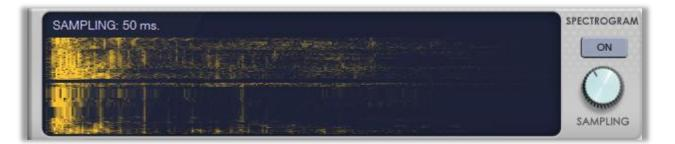
**PCR AnyWhere** has a FFT (Fast Fourier Transform) based spectrogram display to show how the spectral density of a signal varies in time. The waterfall plot is used to show how two-dimensional information changes over time.
