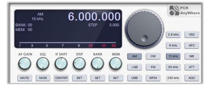
This section contains main display plus controls to tune the receiver, control the audio output, some special receiver functions and memory management.
